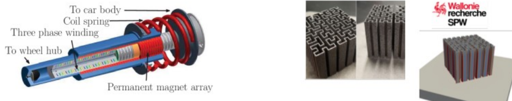
Figure 1: Magnetic actuator design (left) and Fe-Si lattice structures (right) – Cenaero©
